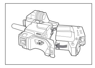
**2** Tighten the CA lock screw to secure the adaptor or transmitter.
